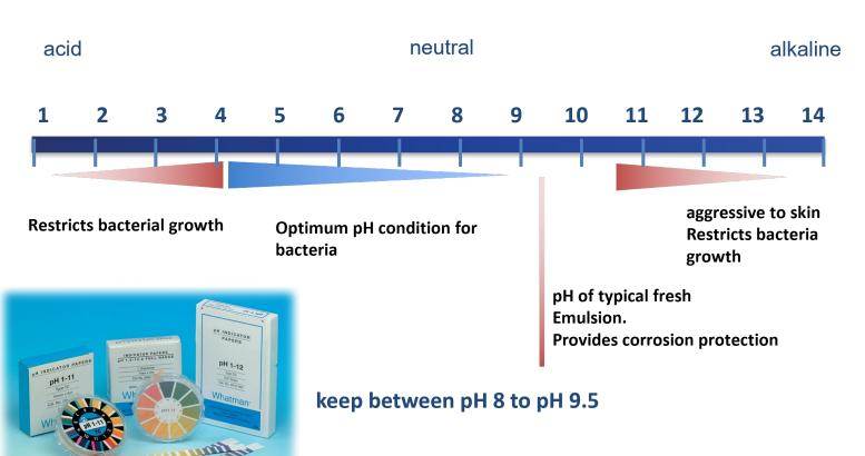
pH measurements give an indication of fluid quality and should always be within the supplier's recommended range.
